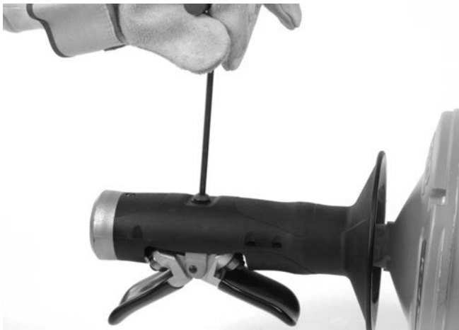
Figure 12A – Removing AUTOFEED Screw
