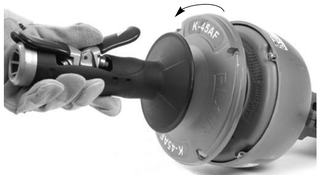
Figure 14 – Twist Drum Apart
