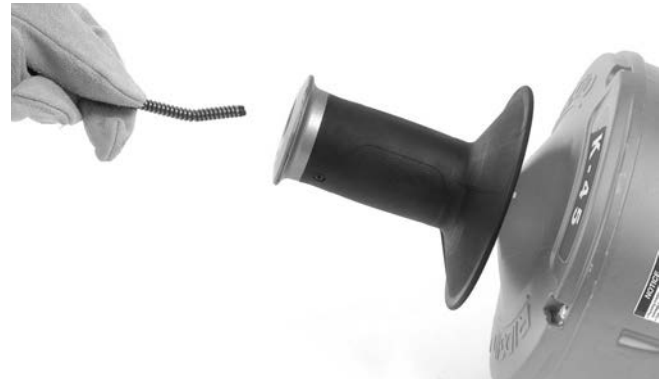
Figure 17 – Loading Cable Without Changing Inner Drum
