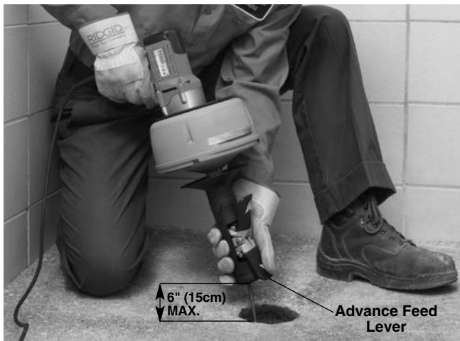
Figure 10 – Feeding Cable With AUTOFEED
