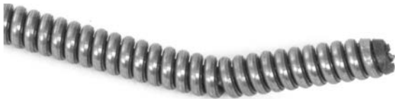
Figure 15 – Bend At Cable End
