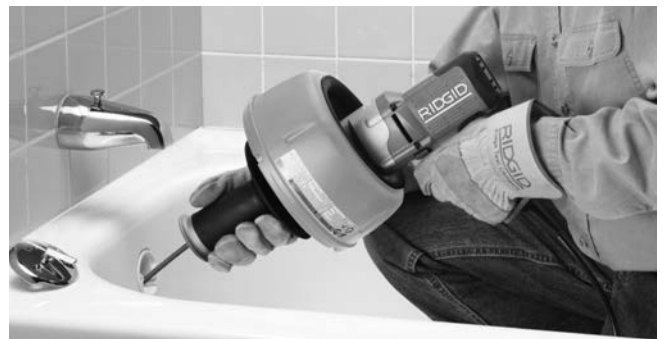
Figure 9 – Push Cable Down Drain Line
