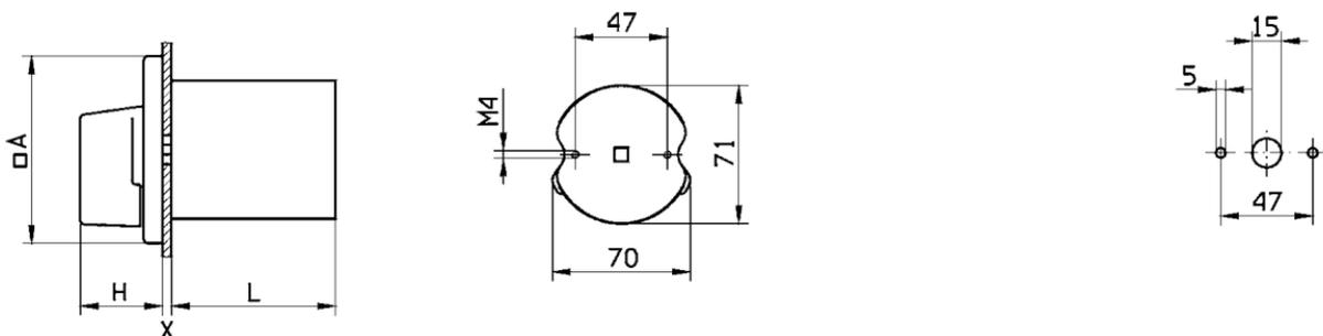
A=96mm, H=44mm, X<sub>max</sub>=4mm, L=105mm
