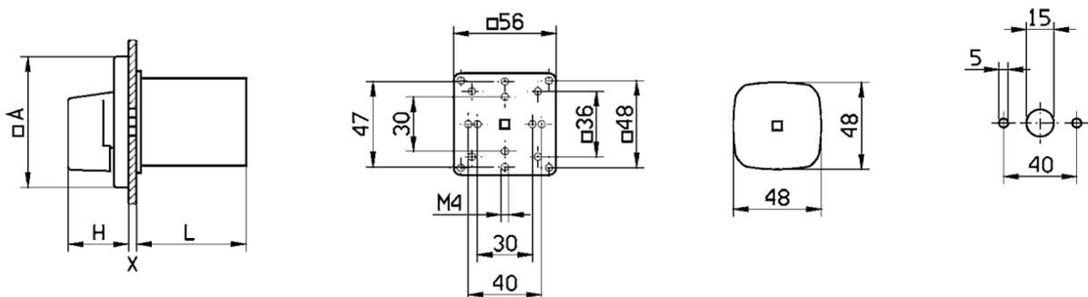
A=72mm, H=34mm, Xmax.=4mm, L=73mm
