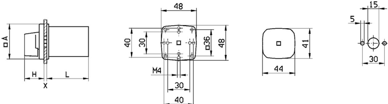
A=48mm, H=27mm, Xmax=4mm, L=33mm
